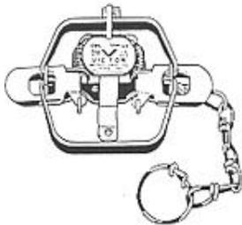
**This is a typical coil spring leg hold trap.** The trap can be released by stepping down on the spring to the left and right of the center pan.
