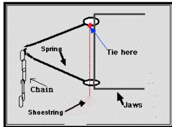
Then, stand on the trapchain, pinning the trap to the ground and haul up on the shoestring. This will compress the spring. Pull and take up the shoestring until both sides of the spring meet. Tie off the shoestring and repeat the process on the other side of the trap, if necessary.
