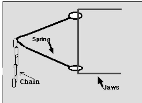
To release the trap, tie one end of a shoestring to the top loop of the spring where it runs along the jaws, run the shoestring through the bottom spring loop and then back through the top spring loop.
